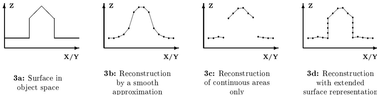
**Fig. 3a-d:** Quality steps of discontinuous surface reconstruction
