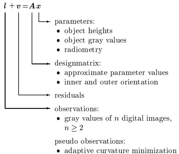
**Fig. 1:** Surface reconstruction with Facets Stereo Vision: observation equations
