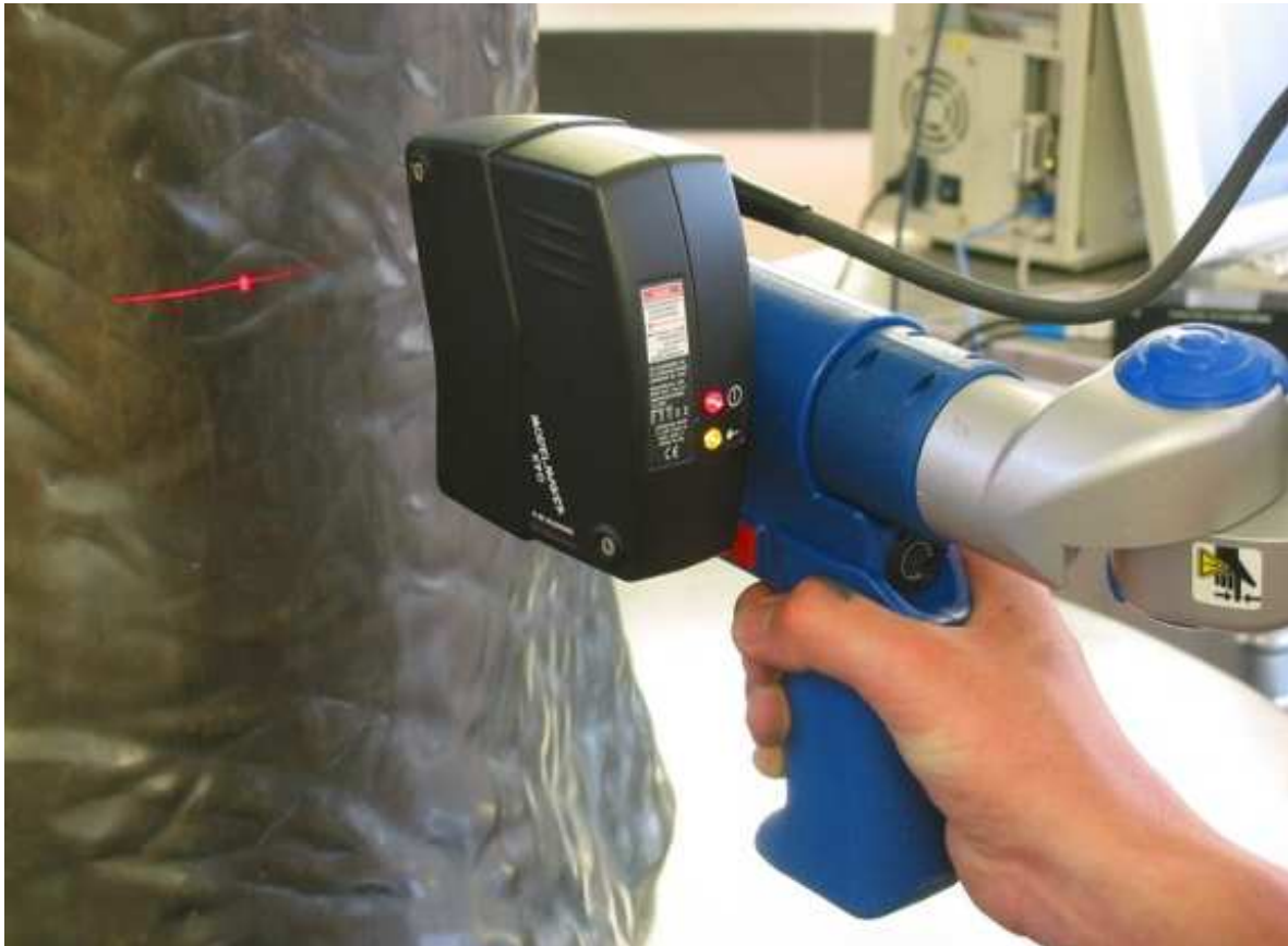
Abb. 2: 3dscanners Modelmaker X70 am 3D-Gelenkmessarm Faro Titanium.
